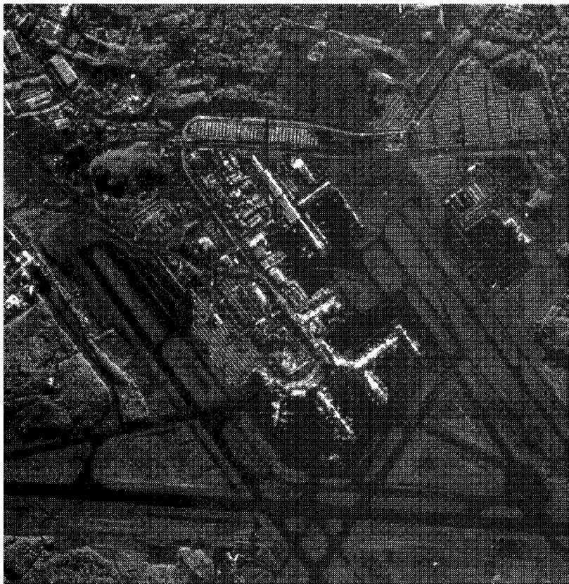
Figure 6. High resolution microwave radar image of the Baltimore–Washington International (BWI) Airport obtained with a microwave SAR modality designed for an unmanned aerial vehicle. The holographic signal processing makes the resolution independent of the sensor’s altitude
