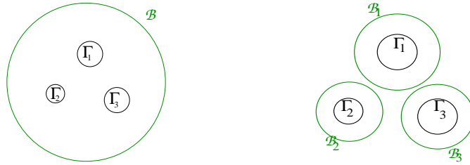
FIGURE 5. Multiple scattering: a single artificial boundary (left) and separate artificial boundaries (right)
