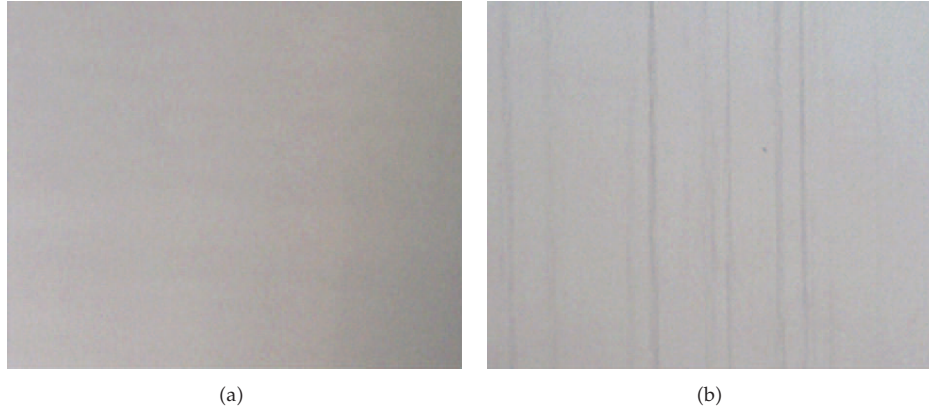
Figure 1: (a) A normal silicon steel sheet; (b) a silicon steel sheet with vertical stripes.
